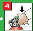
Grab the levers to discharge the fire extinguishing agent from the nozzle.
