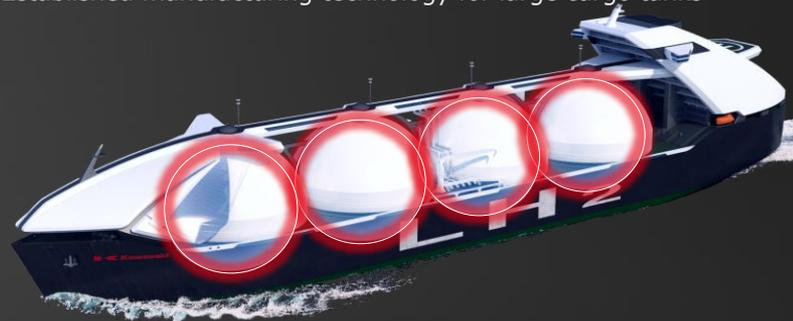
Large liquefied hydrogen carriers are planned to be Zero-Emission powered carriers using boiled-off hydrogen as fuel for maritime transportation.
