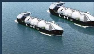
160,000 m<sup>3</sup> x 2 Carriers Cylindrical Tank: 50,000 m<sup>3</sup> x 4 (plan)
