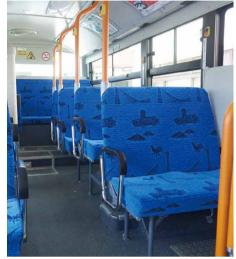
Seats illustrated with various symbols of Kobe, and stanchion poles installed at each seat
