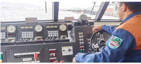
Inside the fourth fireboat Tachibana: the center levers are for operating the water cannon and the pump.
